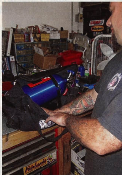
▲ Placement of the 10-pound nitrous bottle (inside an unused duffle bag) is the nitrous system's interior highlight. Stevie bench-builds the setup, first to confirm exactly where brackets must be positioned, and then whether the bag will zip shut once the bottle is secured.
