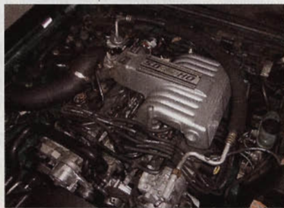
▲ The finished engine looks pretty plain-Jane, doesn't it? Down below, Bassani short-tube headers and a full exhaust system with an X-shaped crossover that includes high-flow catalytic converters and stainless mufflers let out the growl. Now you know the secrets. Try one or try 'em all on your low-buck Mustang project. Hop-up efforts like this are a lot of fun, and they definitely prove that pretty and expensive don't always apply to cool Ponies. 5.0
