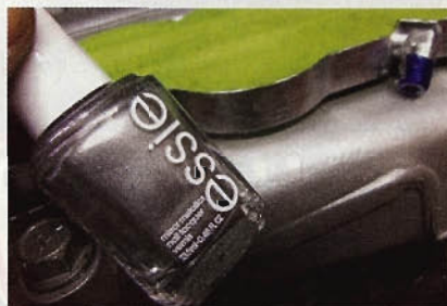
▲ Back under the hood, silver nail polish works great for blending nitrous plates into the flow of EFI upper/lower intake manifolds.
