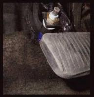
▲A two-step rev limiter is one of three individual rev controllers that are built into Modotek's BlackBox v2.0. Since Cheaper Sleeper is a footbrake 'Stang (dragstrip and stoplight launches done without a transbrake), Stevie mounted a foot-activated momentary button for the two-step on Cheaper Sleeper's brake pedal.
