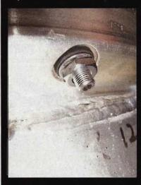
Most NHRA-sanctioned dragstrips require cars with aftermarket racing wheels to use steel valvestems are secured to the wheels with jam nuts. We took that step with our modified 10-holes. A sheared valve stem is the last thing we want to happen when we're racing.
