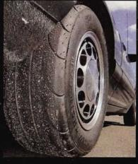
▲ ... And out back, MT's 235/60R 15 ET Street Radials fit perfectly in the Mustang's unmodified (save for fender rolling) wheel wells. One thing to note is the tires are slightly taller than a Foxbody's stock-style boots. As such, fitment might be a concern for aggressively lowered cars and could warrant installing taller rear springs, adjustable control arms, or coilovers.
