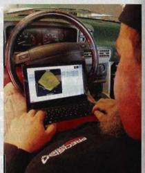
▲ BlackBox v2.0 can present real-time, 3D graphic versions of all tuning tables. Brian feels that this presentation is extremely helpful for novice tuners, as it clearly identifies all of the holes in a fuel or timing map, and helps users build smooth, efficient curves.
