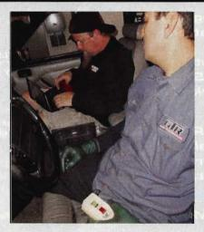
▲While determining Sleeper's power and torque gains were at the top of our must-do list, Brian and Ricardo Topete of GTR High Performance (driver's seat) spent a good amount of time making lowspeed/part-throttle runs on the Dynojet, fine-tuning that aspect of the PCM's calibration.
